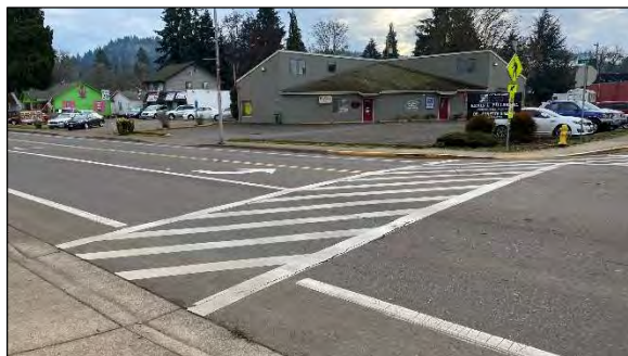
Figure 2-4. Typical Enhanced Crossing on Main Street
